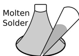
Remove the solder wire from the joint.
