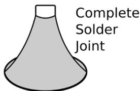
Remove the soldering iron from the joint.
